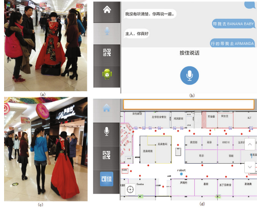
Fig. 8. (a) Talking with customers (b) chatting with app (c) during a tour guide (d) map in the app, red dots are shops, blue dot is robot
