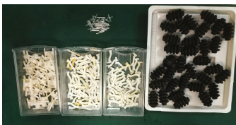
Fig. 5. Soft Robot 3D prints hard components and EPDM (Ethylene Propylene Diene Monomer) airbags.
